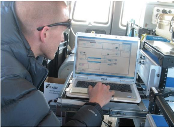
Data from the Mobile Lab's onboard fast-response analyzers are displayed in real time on screens in the van. Scientists in the Mobile Lab look for spikes or large enhancements in the data to identify a source plume and target air sample collection. The multiple compounds analyzed in the discrete air samples will allow scientists to fingerprint various sources in the Basin.
