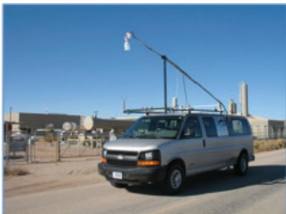
The Mobile Lab is a measurement platform well-suited to study distributed point sources in a contained area like the Uintah Basin. It will be used to map ambient levels of various gases in the Basin and document background levels outside of the oil and gas fields and urban areas.
