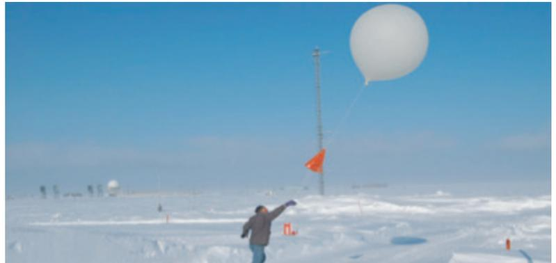
Along with O<sub>3</sub>, the instrument packages attached to the balloon will record temperature, pressure and relative humidity. Similar packages are launched by GMD scientists or collaborators every week in locations as remote as the high Arctic and the Antarctic.
