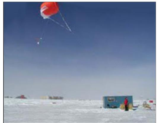
For the Uintah Basin study, researchers launch balloons like this equipped with instrument packages that record data about ozone.
